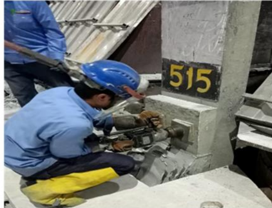
Figure 4. The latest method of tightening the shunt by pneumatic wrench.
